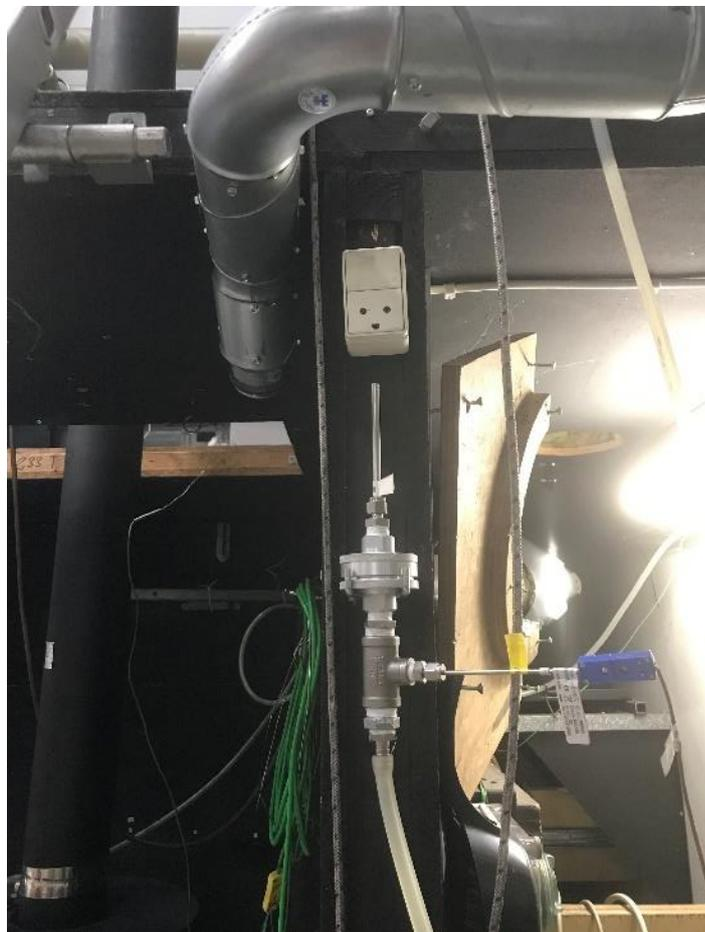
Placement of ambient blank filter holder
