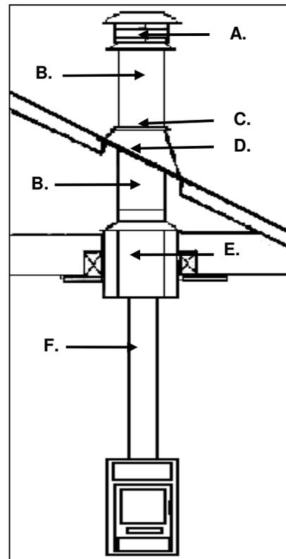
For venting vertically into a Class A chimney, single wall pipe (at least 24 gauge) may be used in the room where the stove is installed. Refer to the manufacturer's instructions for the connection to the listed chimney. The chimney/stove pipe must not be smaller than 6" (15cm) in diameter.
