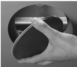
Remove the baffle plate and smoke chikane.
