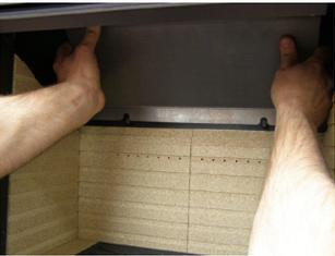
Then remove the smoke impediment by lifting it up and moving it forward. Carefully lift out the smoke impediment.
