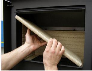
Remove the smoke converter plate by tilting it to one side and turning it a little slantwise. Pull out the plate carefully.
