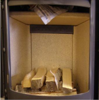
To light the stove, use alcohol briquettes or similar, as well as approx. 2 kg of firewood, split into kindling sticks. Set the air damper to the fully open position.
