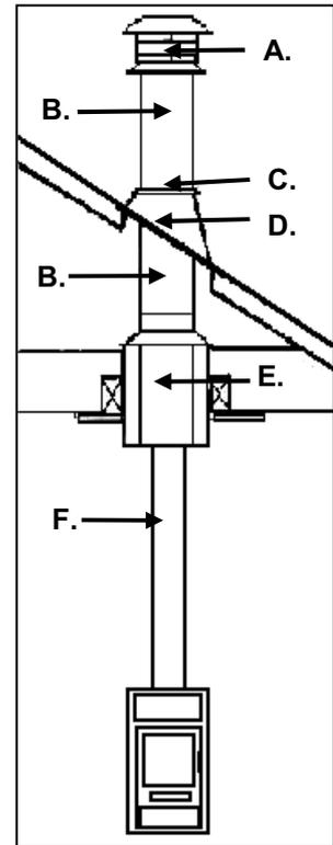
For venting vertically into a Class A chimney, single wall pipe (at least 24 gauge) may be used in the room where the stove is installed. Refer to the manufacturer's instructions for the connection to the listed chimney. The chimney/stove pipe must not be smaller than 6" (15cm) in diameter.
